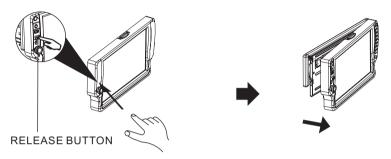
2). Pull-off the front panel and keep the front panel into the case .
